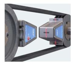
The laser unit emits a laser line that is projected onto the receiver unit. A three-dimensional target area on the receiver unit allows easy detection of the type of misalignment and how to correct it. Belt alignment is achieved when the laser line coincides with the three reference lines on the receiver unit.
